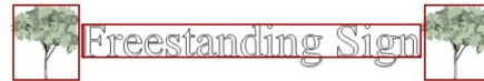
All text included in one rectangle and separate logos included in individual rectangles (sum of all equals sign area)
