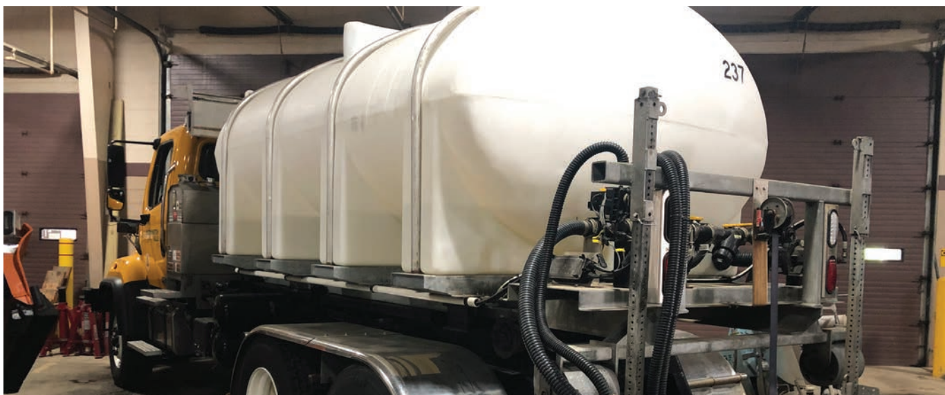
Specially equipped trucks spray the brine mixture onto road surfaces.
